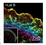
was performed 100X 1.49 NA objective and the Double-Helix (DH) SPINDLE® (Jain et al., 2016; Wang et al., 2017a) module with and phase mask (Grover et al., 2012; Pavani et al., 2009) optimized for far-red dyes.
