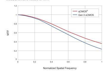
Modulation Transfer Function (MTF) is a type of resolution evaluation. It is the value of how accurately the contrast of an object can be reproduced.
