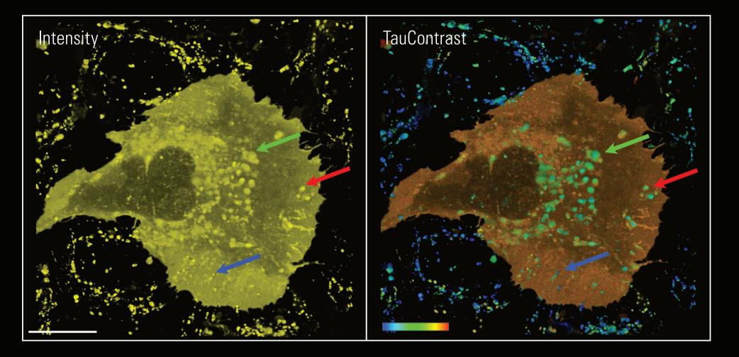
STELLARIS acquires Fluorescence Intensity (Nphotons) and Photon Arrival Times (ns) Simultaneously, resulting in a Average Arrival Time (AAT) image on the fly. The calculations below depict
