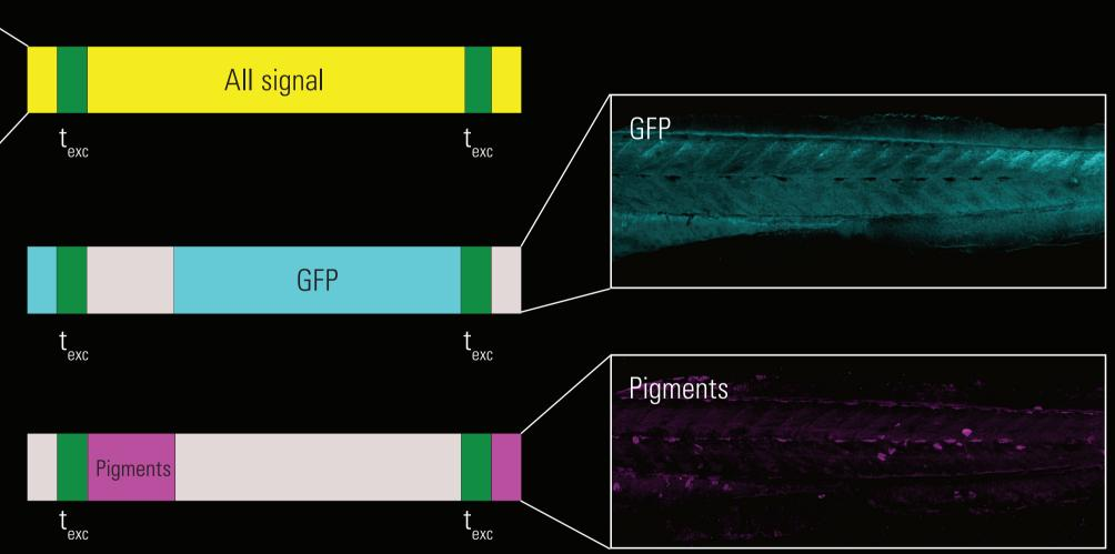
TauScan and TauSeparation allow lifetime-based multiplexing beyond the spectral options with TauSeparation: Separating dyes with overlapping spectra.
