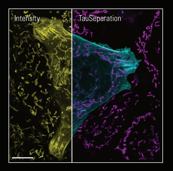
STELLARIS acquires Fluorescence Intensity (Nphotons) and Photon Arrival Times (ns) simultaneously that results in gate-based multi-components graphs. Images can be then separated by selecting the respresenative fluorescent lifetime components
